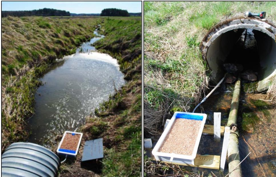
**Figure 2.** Box experiments applied in two agricultural ditches (Kårsta, Vallentuna municipality) to study P removal capacity of filter materials.
