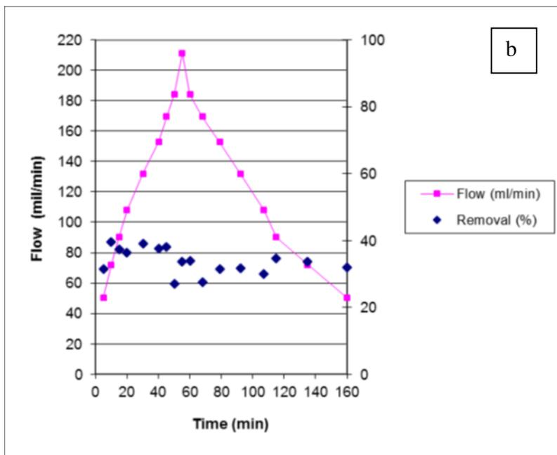
**Figure 6.** Test of the impact of increasing flow on the P removal efficiency. In fig. 6a the dual filter media is new while in fig. 6b the filter has already treated 4000 L of water.
