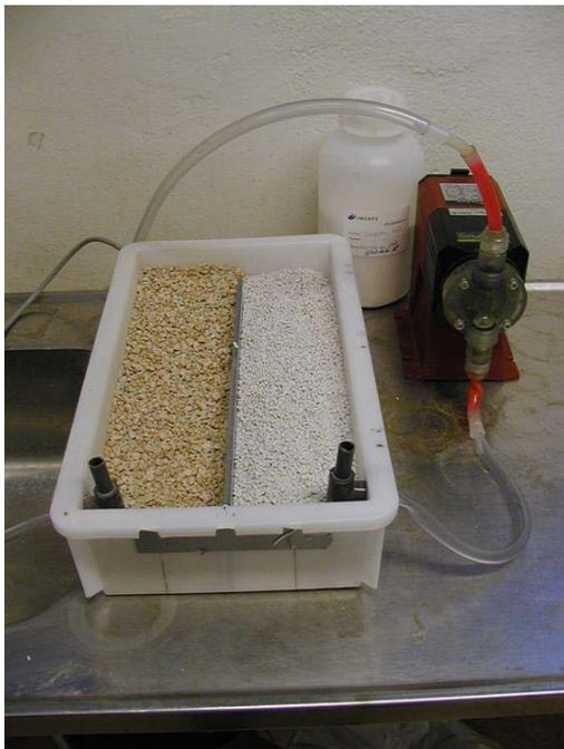
**Figure 1.** Dual filter test with media Sorbulite (right) and Polonite (left). P-solution was pumped to the system with a loading rate of 3 L/hr.
