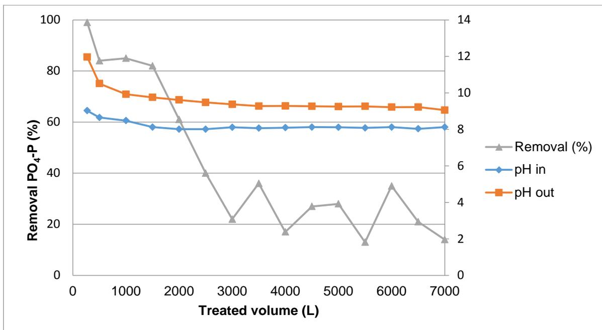
**Figure 5.** Removal of PO<sub>4</sub>-P in dual filter and pH of the influent and effluent water. The water was here spiked with kaolin to simulate the normal turbidity of drainage water (150 NTU).
