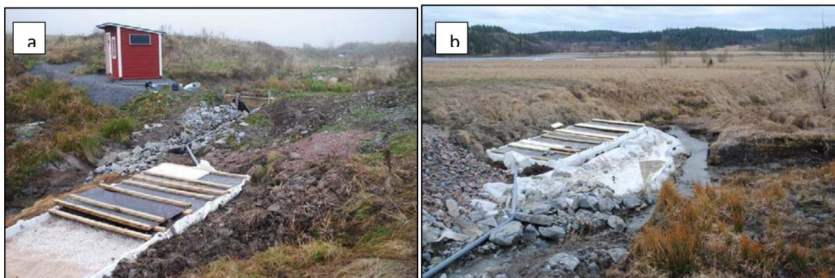
**Figure 3.** Field experiment at Nybble, Jönåker. Ditch water after treatment in a wetland pond is discharged to the filter through a pipe (a). Water treated in the filter is discharged back to the natural ditch.
