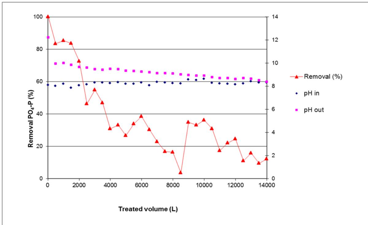
**Figure 4.** Removal of PO<sub>4</sub>-P in dual filter and pH of the influent and effluent water.
