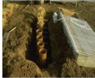
Fig. 4 Lysimeters used in the English study (Fogg 2004). Observed the quality of the biomix showing mainly the unchopped straw.
