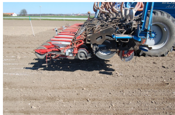
Fig. 1. Seed drill used in trials, 2006-2008. Different levels of pressure can be applied on the press wheel in front of the drill. The disc coulters in front of the press wheel is for application of fertiliser.
