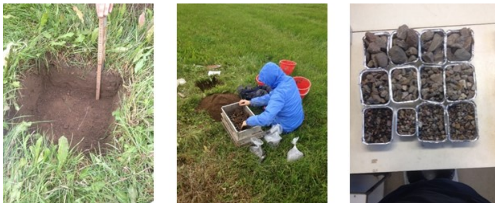
Fig. 1. Excavation and sieving of arable soil (40 x 40-cm quadrats 20-cm depth) disregarding larger stones in situ , and sieving out gravel in the laboratory, obtaining samples for different fractions (> 32-mm, 16- to 32-mm, 8- to 16-mm and 2- to 8-mm) of whole soil. Ekebo site.
