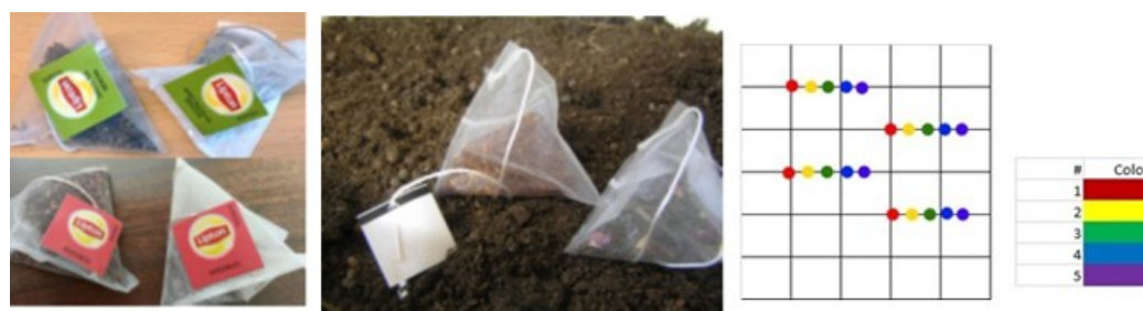
Fig. 2. Tea Bag Index (TBI) measurements made by inserting tea manufactured by Lipton in the topsoil (8-cm depth) of LTEs, using four teabags each of Green tea and Rooibos per experimental unit within a 2 x 2 m grid and retrieving them after different time-periods (15, 30, 60 and 90 days).
