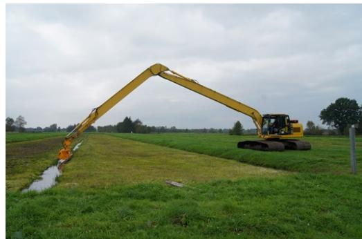
Figure 2: Harvesting of peat mosses without disturbing the farming fields (picture taken in Germany)
